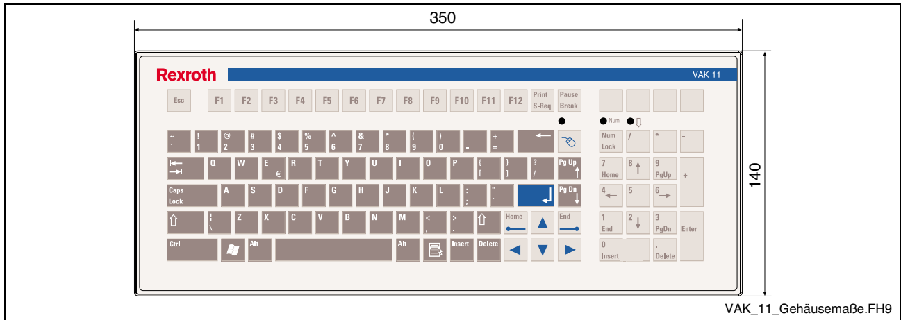
Fig. 7-1: Housing dimensions VAK 11.2
