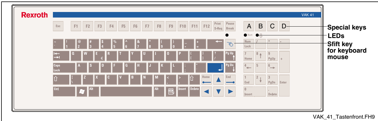
Fig. 5-1: Keypad of the VAK 41.2
